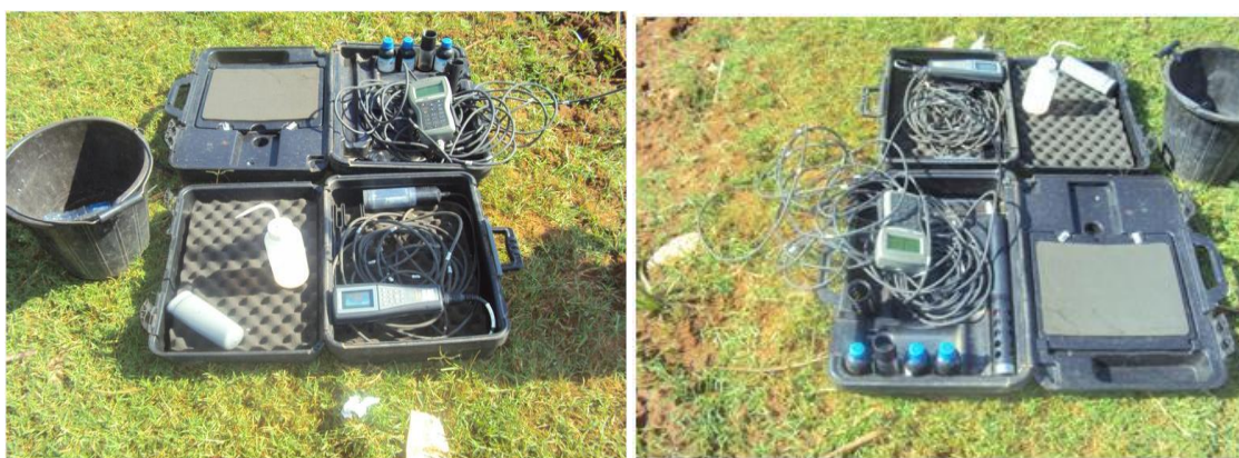
Plate 10. YSI Professional Plus multi-parameter water quality meter
